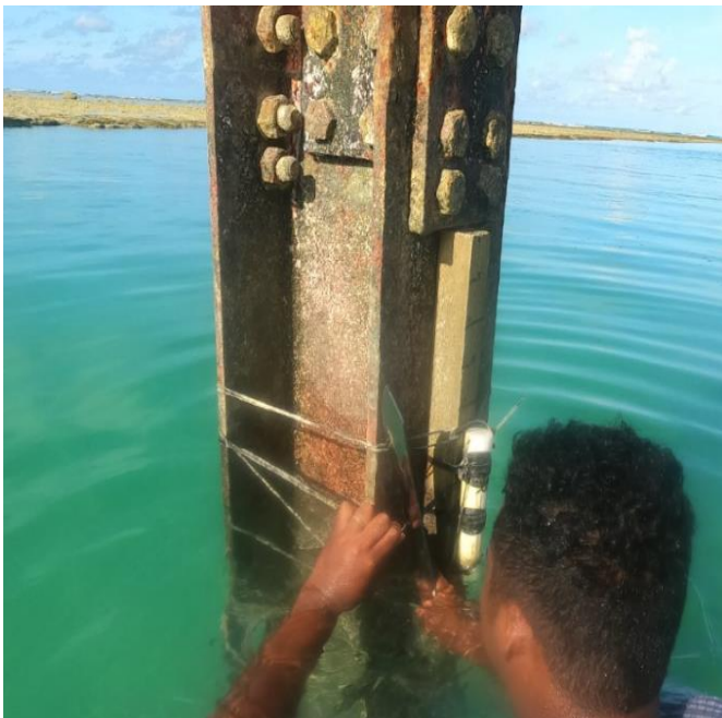
Figure 10: Example of a pressure sensor installation to monitor water levels in Nui, Tuvalu
