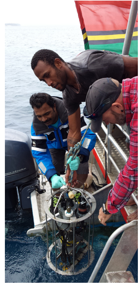
Sampling with the profiler measuring salinity, temperature, light and chlorophyll at depth.
